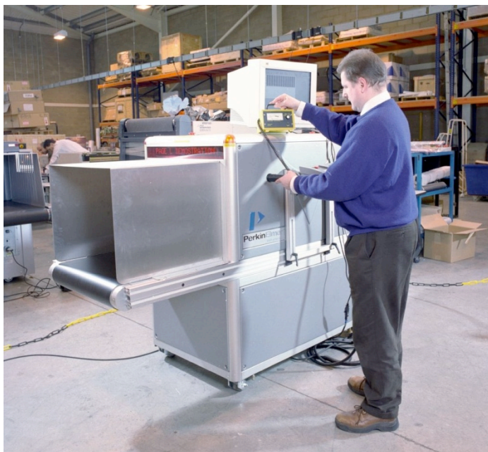
Example of a radiation survey around a baggage inspection unit after maintenance
