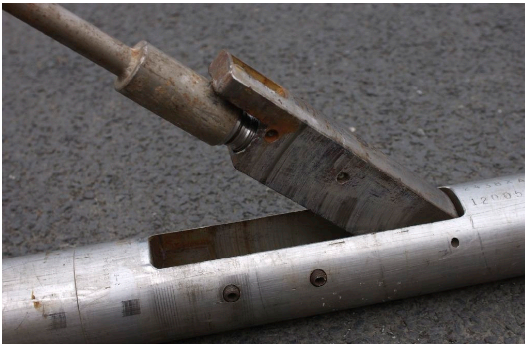
Photograph of source being loaded into a borehole logging tool
